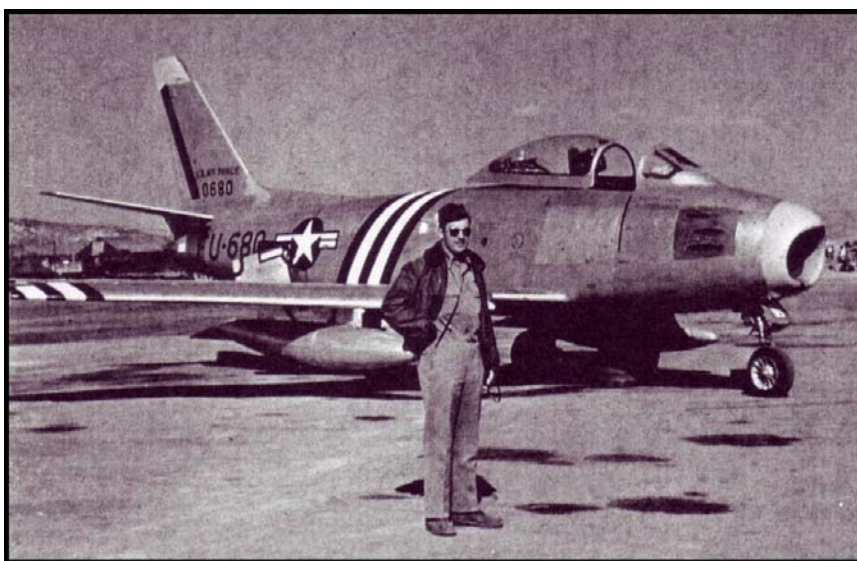
Figure 4 Uncanny picture of F-86E #50-0680 assigned to the 4 th Fighter Interceptor Wing. Lt. Prindle's plane was 50-0681. The "E" model featured a completely moveable tail assembly. The F-86E planes replaced the earlier "A" model in 1951.
