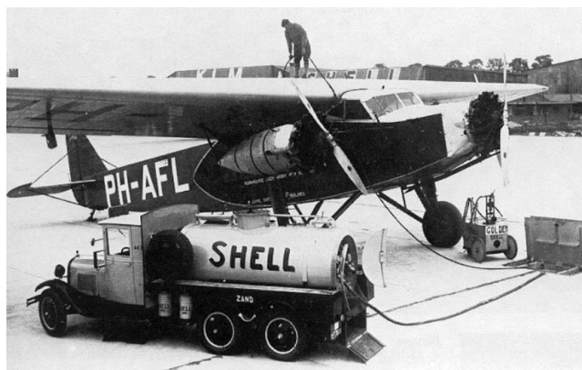
Figure 43 A three-engine Fokker F. XII refueling. With a 900-mile range, the F.XIII could cruise at 120 miles per hour. Source: http://www.dutch-aviation.nl/index5/Civil/index5-2%20F12.html
