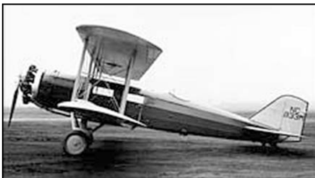
Figure 20 Boeing's 1925 Model 40A mail plane was their first to carry passengers, with room for two people in a tiny cabin, and of course cargo space for mail. Twenty-four of the mail planes built were ready to fly on July 1, 1927, when they assumed the former trans-continental route between San Francisco and Chicago.
