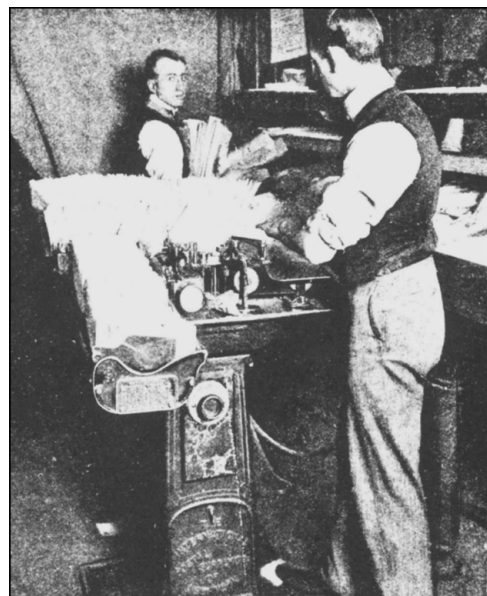
Figure 15 Photo of the seven-bar Hey-Dolphin International machine canceller in operation.
