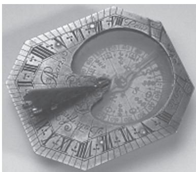
Figure 4 This classic style ca. 1780s Butterfield portable sundial (made for 200+ years) could keep travelers up to speed on local sun time and thus keep to a schedule.
