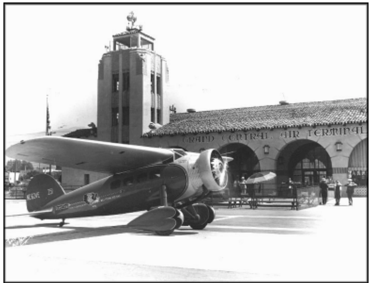
Figure 6-1 The Lockheed Vega 5, shown in this illustration was one of the faster, early 1930s commercial airliners. This particular aircraft, No. 251, was the personal aircraft of the Transcontinental and Western Air, vice-president, Jack Frye. Note the addition of an engine cowl and streamlined pants over the wheels, an early development that increased speed and engine cooling substantially. Insignia shows the old Western Air Express, Indian warbonnet, and the nose carries the words, Transcontinental and Western Air, Inc. Below the cockpit is "U. S. Mail, AM 34," denoting the CAM (Contract Air Mail) route. (courtesy Philip S. Docktor)
