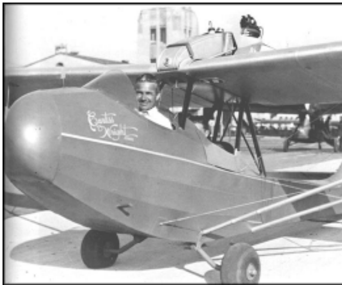
Fig. 5-8 Major Corliss C. Moseley is seated in a low cost, two seat, tiny aircraft, after setting a slow-speed record by flying the plane around the field at a speed of only 25 mph. The aircraft, called the "depression baby," was a 45hp Curtiss-Wright CW-1 Junior. It was an attempt by Curtiss-Wright to provide an aircraft that was inexpensive to own and to fly. (Courtesy of the Grand Central Company)
