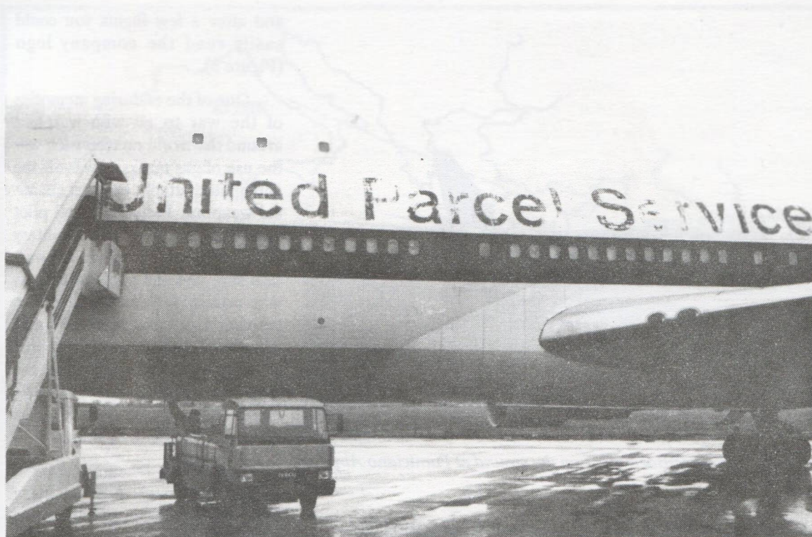
Figure 3. This photo, taken at Fumicino Airport, reveals the cheap brown paint completely worn away, taking some of the original UPS lettering with it.
